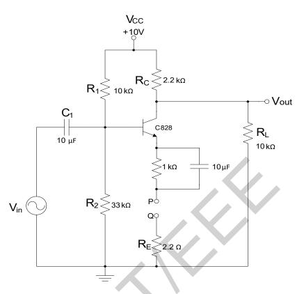
Fig 4.1: Study of current series feedback amplifier.
